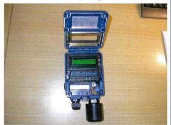
Electrical connections for the power and signal are made to screw type terminals mounted on the Output PCB.
