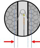
**2.** Using the integrated installation hook, hang the device as close to the bore hole as possible. Ensure the yellow plastic installation strip is left in place. Remove the wire reel for anchor 1 and allow to unspool.
