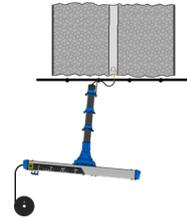
**3.** Using installation rods, push anchor 1 into the bore hole to the required height. Repeat steps for anchor heights 2, 3 and 4 (where applicable). Seat spring anchors by pulling down on each wire placed into the bore hole.
