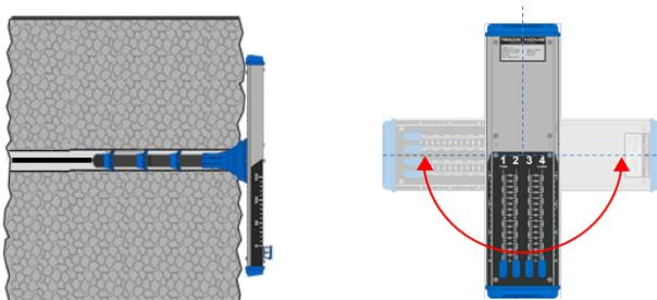
**Sidewall Mounting Orientation**
