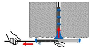
**Note:** Device orientation will be dependent on local strata conditions and should be determined on a case by case basis. Use of the side scale for viewing at distance requires telltales to be mounted perpendicular to the roadway.
