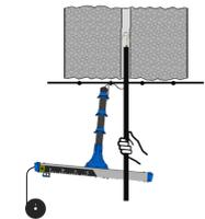
**4.** Unhook the device and insert into the bore hole. Take care to push the unit from the centre into the bore as far as it will go. Pull the slack cable through the device from the back end as you do this.
