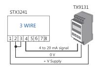
The sensor may be connected the 3 or 4 wire connection mode.
