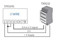
A low impedance two-wire voltage output signal requiring a separate power supply to the sensor. This can be derived from a Trip Amplifier or Programmable Sensor Controller, when one of those is used as the monitoring instrument.
