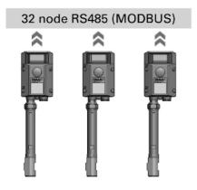
communicate with the master unit on a single data cable.
