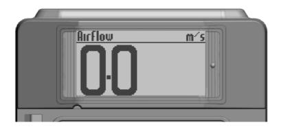
After five seconds the **Main Display** will appear. The **Main Display** displays the current airflow.
