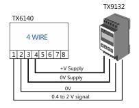
This connection configuration works well up to about 100 metres distance between the sensor and the monitoring equipment.
