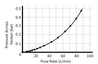
Response characteristic of a venturi system in a Ø25 pipe. FLOW UNITS (Differential Pressure)
