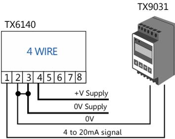
The sensor can also be operated in the 3 or 4 wire mode using a separate power supply.
