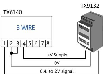
A low impedance two-wire voltage output signal requiring a separate power supply to the sensor. This can be derived from a Trip Amplifier or Programmable Sensor Controller, when one of those is used as the monitoring instrument.
