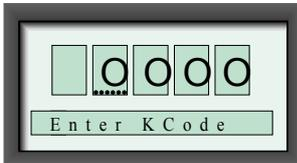
This entry screen will only show if an active keycode has been set. If the entered keycode is accepted, the display moves on to the MENU section. If the entered keycode is invalid, the display returns to the normal measurement mode.
