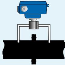
One of the three FLOW measurement units may be selected where a TX6143 series Differential Pressure Sensor is installed across an orifice plate or venturi to monitor flow velocity.
