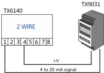
The output signal from terminals 1 and 4 is a conventional 4 to 20 mA two wire current regulated signal loop.
