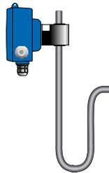
The sensor will tolerate reasonable levels of contamination and foreign particles present in the process medium but where conditions are particularly aggressive, the sensor should be protected with a U-bend or an isolating seal.
