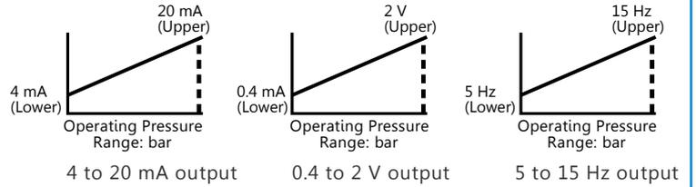
The various parameters of the signal scale and display values can be *modified* to suit the individual characteristics and imperatives of a particular installation or process.
