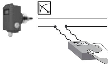
Check at regular intervals, that the value of the output signal agrees with the value of the display reading. Re-calibrate if necessary.
