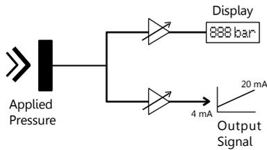
The scaling of the output signal and the corresponding value of pressure presented on the display of the sensor is accurately calibrated, in bar, during manufacture.
