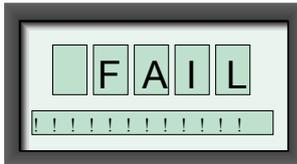
The processor will constantly carry-out a self-test routine of the main circuit elements; EPROM, memory, comms and display read/write function.
