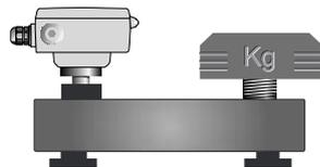
Under normal circumstances, the calibration of the actual pressure capsule will not change by any significant degree. Check the accuracy at least once per year by comparing the display reading with an accurate standard.
