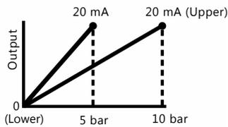
The sensor may be installed in an application that requires a lower operating pressure range than the standard *calibrated* range (e.g. 5 bar utilisation on a 10 bar full scale sensor).
