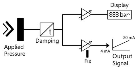
The scaling of the output signal and the corresponding value of pressure presented on the display of the sensor is accurately calibrated, in bar, during manufacture.
