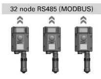
Up to 32 sensors acting as slaves can communicate with the master unit on a single data cable.
