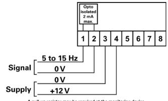
A pull-up resistor may be required at the monitoring device
