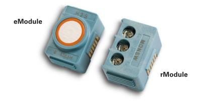
Sentro eModules are used for environmental gas concentration monitoring. Three types of eModules are available (detailed on page 4): electrochemical cells to detect toxic gases, catalytic combustion sensors to monitor flammable gases and infrared sensors to monitor Carbon Dioxide or Methane in the environment.
