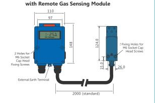
3.2 TX6383.84 Flammable Gas Sensor/Transmitter
