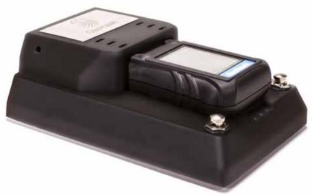
Rapid and convenient gas response testing of Gashawk prior to deployment. Equally suitable for individual users or multi-user validation checks.
