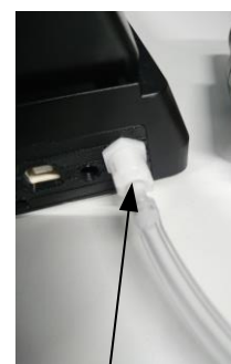
Lock onto UDS connector (turn until it clicks). Gas flow then activated
