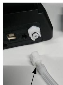
Push fit barbed connector onto 1/8" ID tube.
