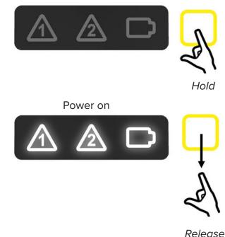
3. The XD One will perform a self test routine to check the sensor element, electronic circuitry and battery health.
