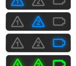
On initial power up, the XD One will perform a self-test sequence indicated by a sequential blue flash of each icon.
