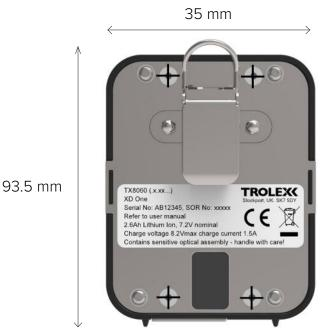
The XD One is supplied with a stability bracket and strap for additional support of the product when body-mounting. Fit the bracket using the bottom two threaded M3 mounting holes and the fixing screws provided.
