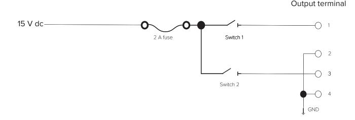
Equivalent circuit if powered from a mains voltage.
