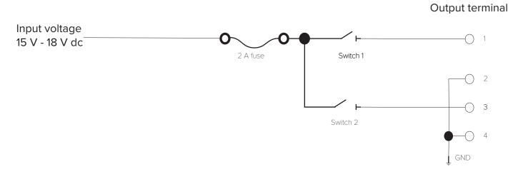
Equivalent circuit if powered from a dc voltage.
