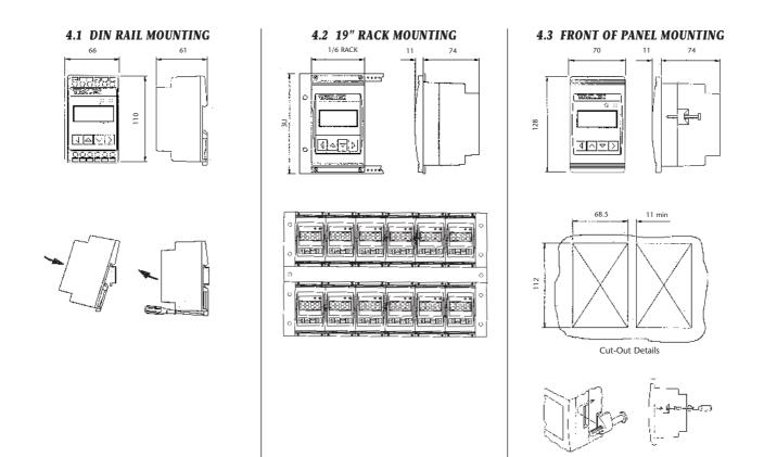
NB: The front of the panel seal is environment proof to IP65, enabling the module to be used in outside operating conditions.
