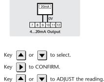
The display value shows a representation of the pulse width modulation generated by the internal processor to produce the analogue output signal and can be used as a guide depicting the increase/decrease of the signal during adjustment.
