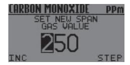
Press **R** to continue with the normal span calibration (previous page)
