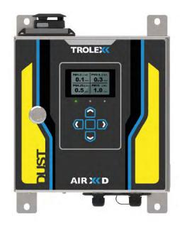
The **AIR XD** uses an innovative Optical Particle Counter (OPC) that combines adaptive particle flowrate with advanced sensing technology to ensure a high level of measurement accuracy. The size of each particle is instantaneously measured and classified at up to 10,000 samples per second to allow detailed real-time reporting in high dust environments.
